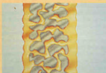
Figure 2—A schematic of the internal Captek™ structure shows a matrix of 97% gold reinforced with small particles of a very high fusing and high strength platinum/palladium/gold alloy.
